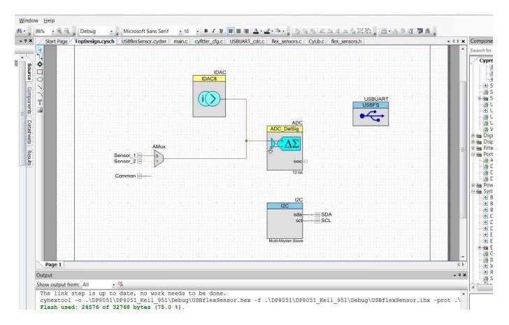
The schematic capture tool inside PSoC Creator is used to configure the PSoC. The USB kit uses the IDAC to source a current to ground through either Sensor 1 or Sensor 2. The ADC measures the voltage across the sensor. The voltage that the ADC measures is determined by ohms law:
