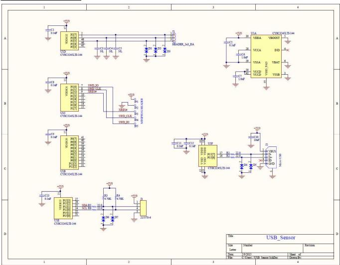
The heart of the USB kit is the Cypress PSoC CY8C3245LTI-144. The Cypress PSoC is a great part to use with Flexpoint Bend Sensors since they have an integrated current DAC. This allows the Bend Sensor® to be interfaced with the ADC directly without the need of any external components like voltage divider resistors or op-amps.
